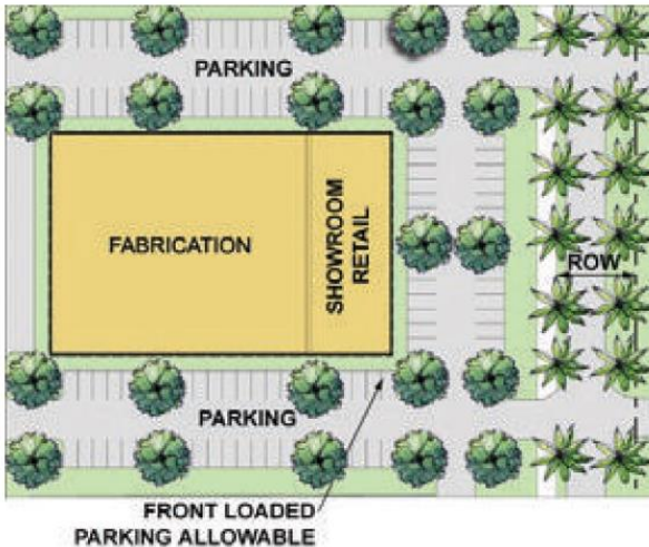
Building with parking in front, side, and rear setback.
